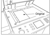
When copying originals with high transparency, such as OHP films and tracing paper, place a blank sheet of paper the size of the original or larger over the original.
